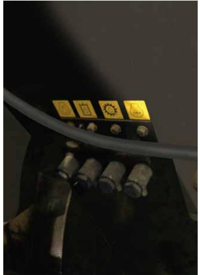
All pressure taps and sight gages are easily accessible. Fluid drains provide environmentally friendly drainage capability and are grouped together for convenient serviceability.
