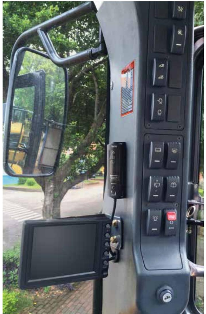
All-around visibility is supported by a rear view camera acting as an extra eye on the jobsite.
